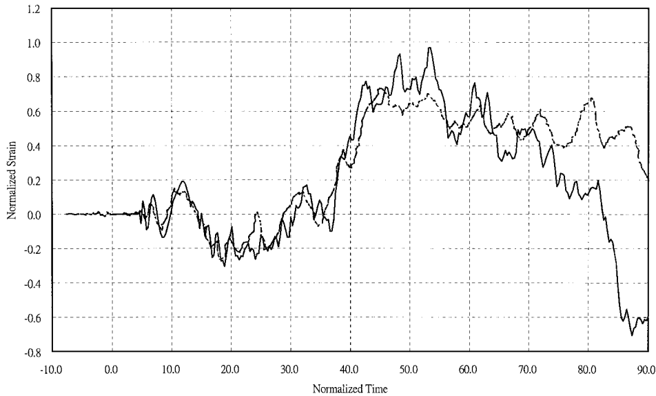
Fig. 10 Comparison of the theoretical value and experimental data for the bending strain in member 6-7: —, theory, and ···, experiment.
